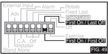
The Off / Exercise DIP switch selects whether or not the control is to exercise the primary pump and boiler pumps (FIG. 50). If the DIP switch is set to Exercise, the pumps are operated for 10 seconds after every three days of inactivity.
